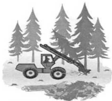
A one-grip harvester cutting a spruce stand for regeneration and bunching of forest residues .
